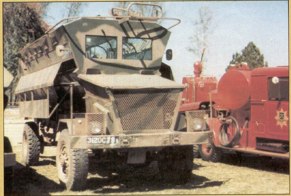
Front view of Hippo. Note machine-gun mounting, and what I can only assume is a wire cutter or deflector.
