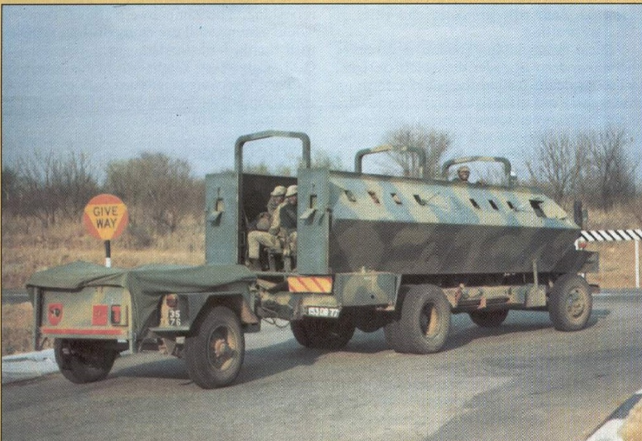
Rear view of the Crocodile towing a stores trailer. Note the water tanks behind the rear wheel and the rear doors with rifle ports.
