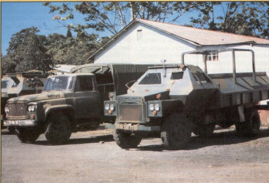
Army Puma showing protected cab and cargo body. Behind the Puma is a Nissan GS truck and both these vehicles were photographed at the School of Infantry, Gwelo. Crew: 12 troops, one driver and mine/ambush sentry. There was a version of the Puma which was fitted with drop sides, but in practice these were rarely used. This vehicle had a different cab to the normal Puma.
