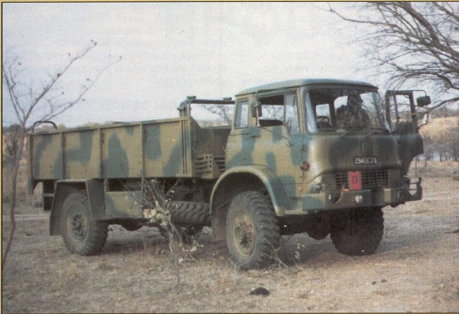
Bedford MK (4x4) 4000kg GS truck, purchased or on loan from South Africa. I believe this was taken in 1978 and belonged to 2 RR.
